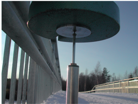
Fig. 15. Displacement gauges used on the western and the eastern sides of the bridge; (a) shows the test setup with gauge, weights, steel wire, and tracked wheels for the wire; (b) shows where the gauge is in contact with the weight underneath it
