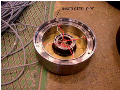
Fig. 5. Earth-pressure cell used for monitoring
